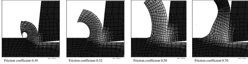
Figure 1: Friction Coefficient Sensivity Analysis
