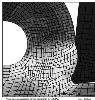
Figure 2: Von-mises stress using a craterized tool
