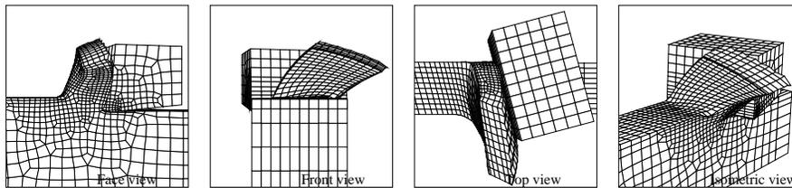
Figure 3: 3D Representations of the Oblique Cutting
