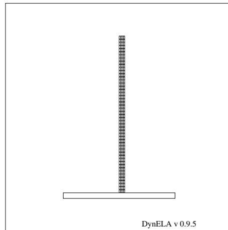
Figure 4: Initial mesh used for the thin walled cylinder under uniaxial compression
